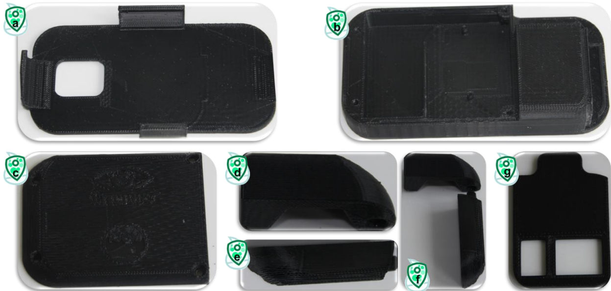
Fig. 4: All elements printed by the 3D printer: a) Smart phone holding element, b) Cuvette and electronics holding element, c) Lid for electronics part to fix with screws, d) Lid for cuvette, e) Cover for LEDs, f) The way to combine the lid for the cuvette and the cover of the LEDs, and g) Filter set up. Image courtesy Anna Friedrichs.
