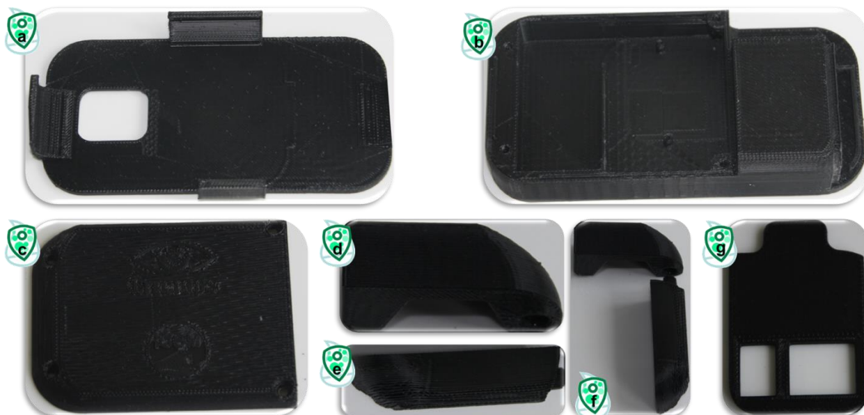
Fig. 12: All elements printed by the 3D printer: a) Smart phone holding element, b) Cuvette and electronics holding element, c) Lid for electronics part to fix with screws, d) Lid for cuvette, e) Cover for LEDs, f) The way to combine the lid for the cuvette and the cover of the LEDs, and g) Filter set up. Image courtesy Anna Friedrichs.
