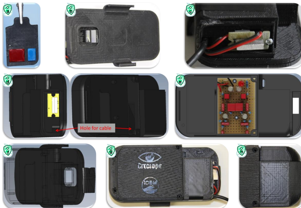
Fig. 15: Image-by-image instruction to build the smart phone adapter to measure algal fluorescence in water: How a) to glue the filter set up, b) to position the mirror, c) to fix the LED set up in to the 3D-element, d) to place the cables, e) to position the circuit board, f) to combine the smart phone holding element (dark) and the prepared cuvette and electronics element (shadowed), g) to place the lid of the electronics and h) to place the lid of the cuvette and LED. Images d), e), and f) produced with e-drawings. Images a), b), c), g), and h) courtesy Anna Friedrichs.
