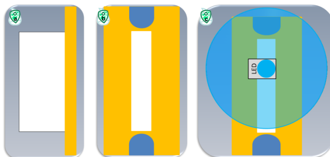
Fig. 14: Schematic view of the LED set up: aluminium plate (white) and breadboard (orange). a) Side view of the LED set up, b) Front view (including holes for screws), and c) Front view with glued LED (including light cone).
