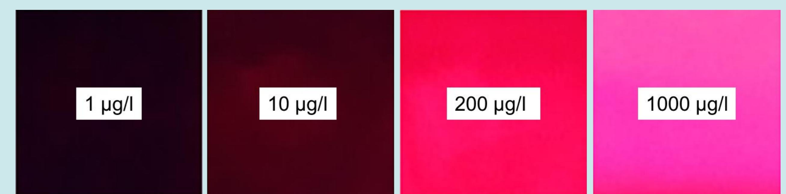
Fig. 6: Examples of selected squares of RGB images for the given Chl a concentration.
