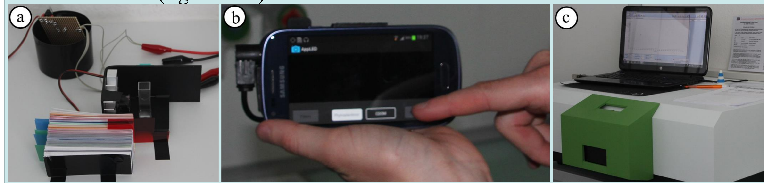
Fig. 4: Measurements with the (a) set up for proof of principles, (b) prototype and smart phone application, (c) control measurements
